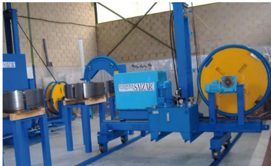
The head has a hydraulic element to pull the strap. This means that **the strap can be tightened at the customer's chosen pressure** (right up to breaking the strap if necessary).
